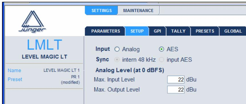
Here you can choose the used input. If AES is chosen, the Level Magic LT synchronizes to the digital input. If you use the analogue input you have to choose if you want to work with the internal SYNC 48 kHz or with an external taken from the AES input.
